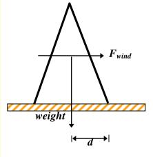
The force from the wind acts in the center of the left board, causing a tipping torque of
