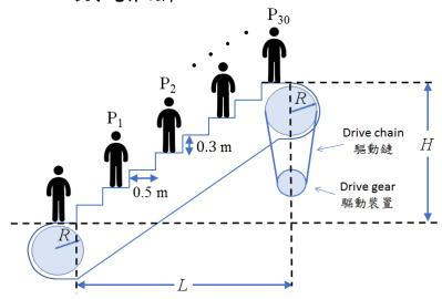
An escalator has a horizontal length L=30 m and a height H=18 m. It transports passengers upward through its length in 90 s. Each step on the escalator is 0.5 m deep and 0.3 m high. There are 60 steps on the escalator.
