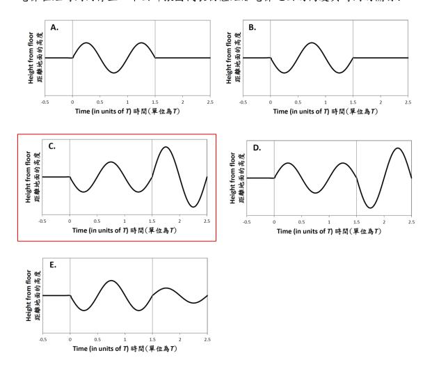
At t = 0, the upward acceleration produces a downward fictitious force. The downward force in a short time produces a downward impulse setting the mass to oscillate downwards. At t = 3T/2, the upward deceleration produces an upward impulse, further increasing the velocity of the mass.
