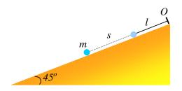
(a) Note that the particle is momentarily stopped at its lowest position. By the conservation of mechanical energy, the loss in gravitational energy becomes the gain in the elastic potential energy.
